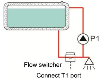
Tap seems like a remote controller, it controls the running of DHW pump. This control mode of DHW pump is an energy saving solution.
