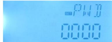
Through password set to limit the user to change some parameters, 4 digitals needed. Default is 0000
